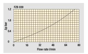
The curves are plotted using mineral oil with density of 0.86 kg/dm<sup>3</sup> in compliance with ISO 3968. ∆p varies proportionally with density.
