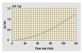
The curves are plotted using mineral oil with density of 0.86 kg/dm³ in compliance with ISO 3968. Δp varies proportionally with density.
