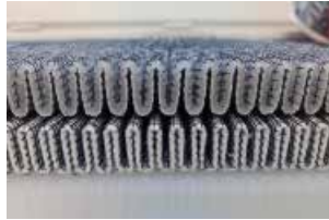
The Filter Media has absorbed water
